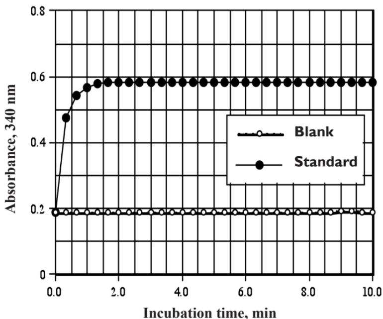
**Figure 1.** Increase in absorbance at 340 nm on incubation of 20  $\mu\text{g}$  of D-malic acid with hexokinase and glucose 6-phosphate dehydrogenase in the presence of  $\text{NAD}^+$ .
